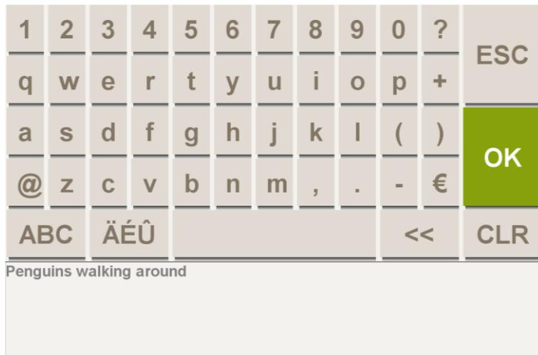
Pressing *OK* overwrites the old setting with the new text. *ESC* dismisses the new text and keeps the old setting. To clear the whole line, press *CLR*. The << button clears the last character that has been entered.
