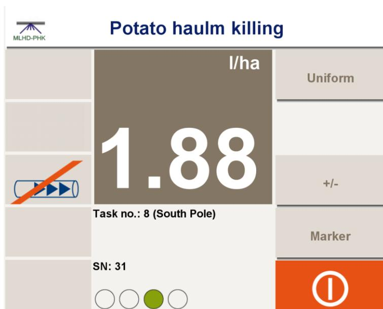
The main menu bar changes and a moving green indicator appears. Calculated application rates are continuously sent to the sprayer controller and all relevant data is logged to the log-file that is linked to the selected task. The main menu bar displays the following options:
